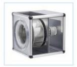
With regard to the GigaBox T120 series, the motor is located outside of the air flow and it is separated from the impeller by a thermally insulated wall. The motor-impeller unit can be removed without dismantling the duct system.
